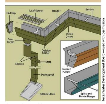
Figure 4. Gutter and downspout components.
