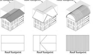
Figure 3. Sizing the catchment area of a roof. Notice how differences in roof slope configuration and shape do not change the catchment area.
