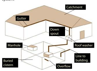
**Figure 2.** Underground rainwater collection and storage system.
