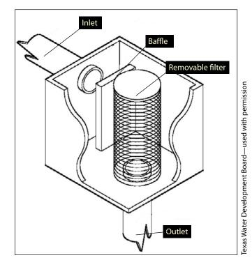
Figure 8. Illustration of a roof washer filter system that cleans rainwater before it enters the storage tank.
