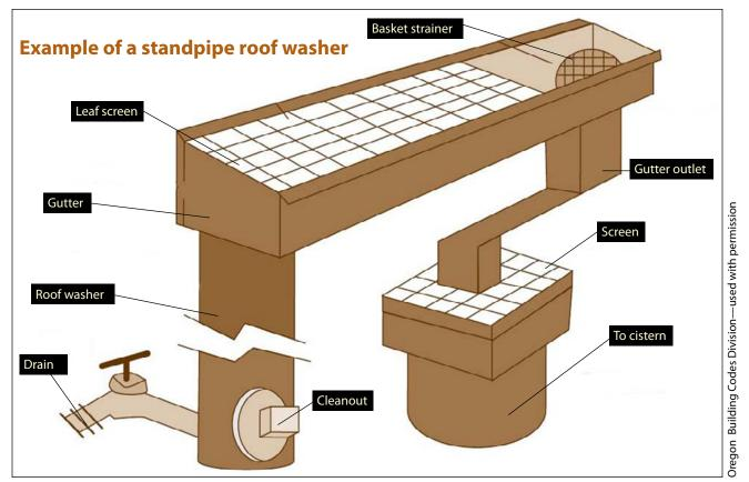
Figure 6. Rainwater collection arrangement showing position of PVC standpipe roof washer or first flush diverter.
