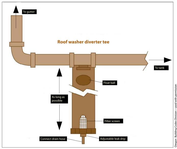
Figure 7. PVC standpipe first flush diverter components.
