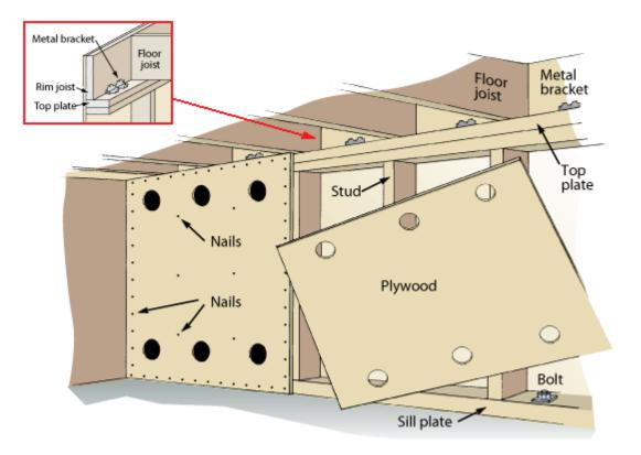
This cutaway diagram shows how weak cripple walls can be strengthened by properly attached plywood sheets.
